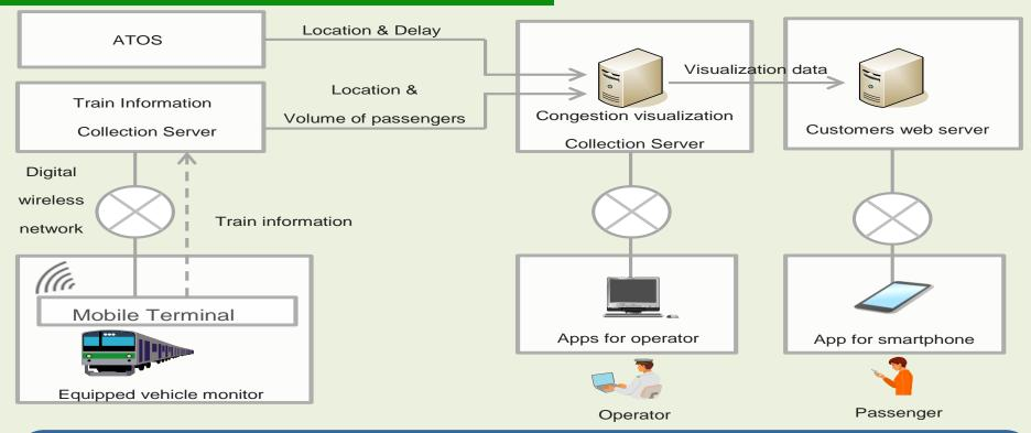
We use data on train location, delay time, and passenger volume in this study. This data is obtained from an existing system, namely a traffic control system (ATOS) and train data collection server.
